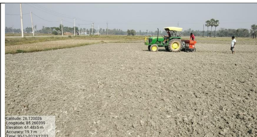
Wheat Sowing with Zero till cum fertilizer machin
