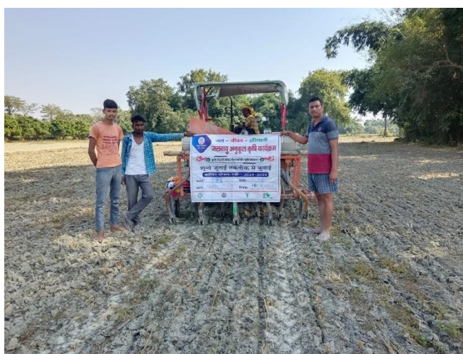
Sowing of Wheat Variety - (HD-2967) by zero tillage technique at Village- Balwa-bariya under CRA Program KVK Piprakothi, East Champaran.
